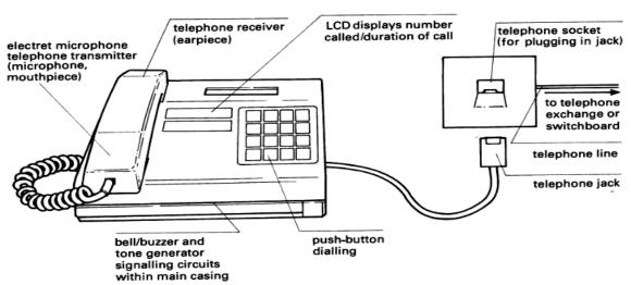
typical push-button type telephone (faster dialling using buttons, which code dialled digits into voice frequency tones to signal destination number).
