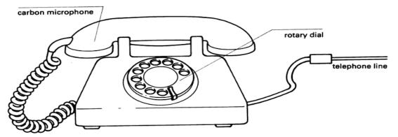
older type telephone using rotor dialling, which generates pulses to code digits defining destination
